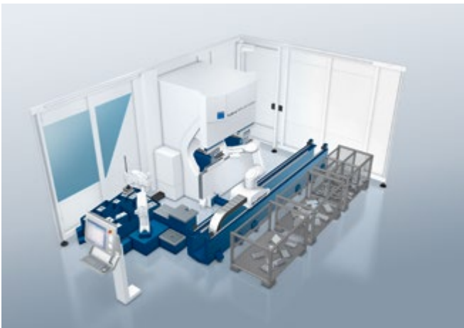
TruBend Cell 7000 with BendMaster (15) and LoadMaster.
