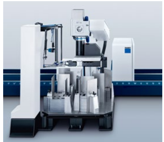
Sheet removal station with rotary table
