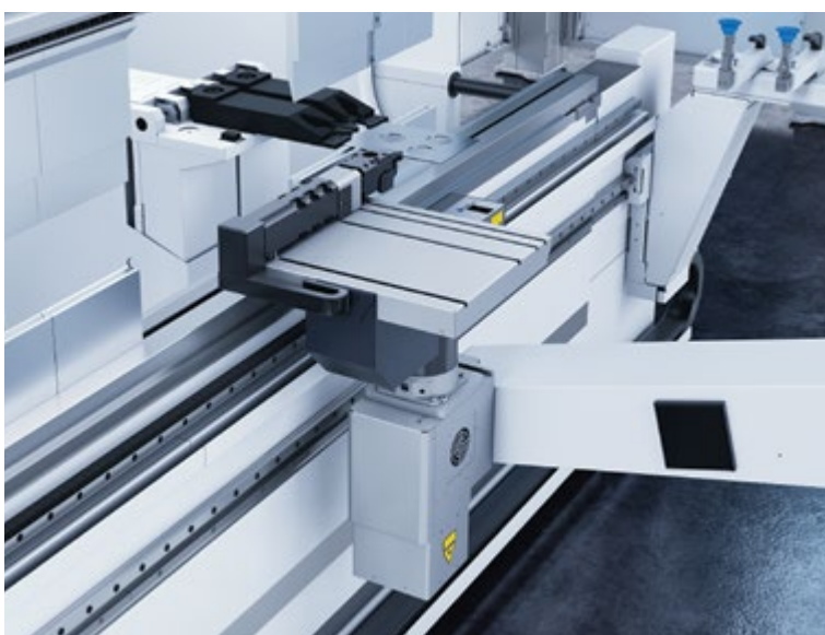
Pivoted-jaw gripper with moving and rotary axis
